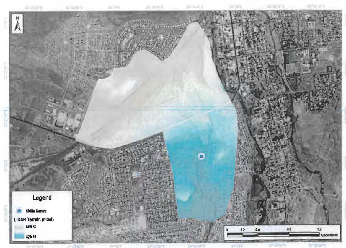
Figure 4-1: The DTM that was used for the HEC-RAS 2D hydraulic modelling overlaid on a satellite view of the area
