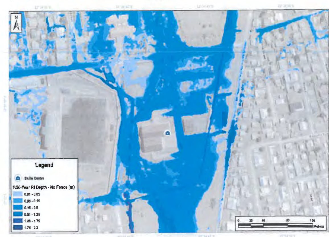
Figure 4-18: Flood inundation depths for the 1:50-year RI flood event assuming no obstruction at the fence (free flow conditions)
